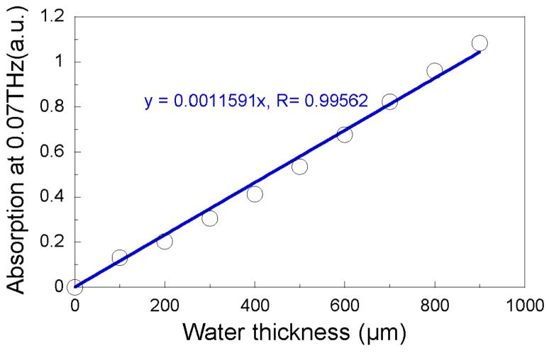
Good correlation between water thickness and THz absorption at 0.07 THz.
