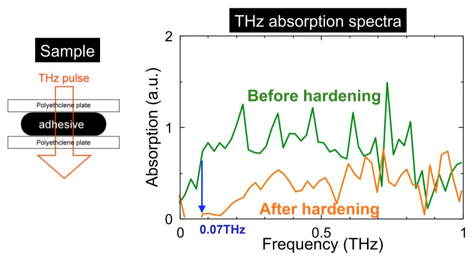
Difference of THz absorption spectra before and after hardening of the adhesive is obvious.
