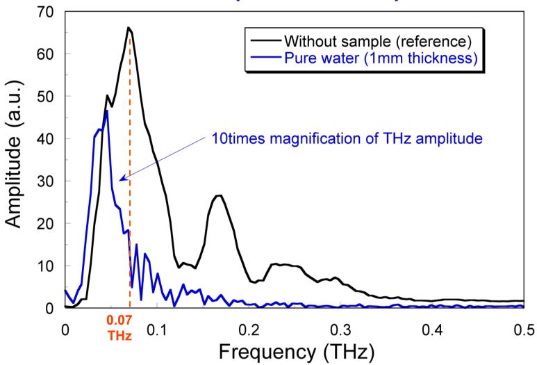
THz wave over 0.1 THz is disappeared by broadband, strong absorption of water. THz absorption at 0.07 THz is used for quantification of water content.
