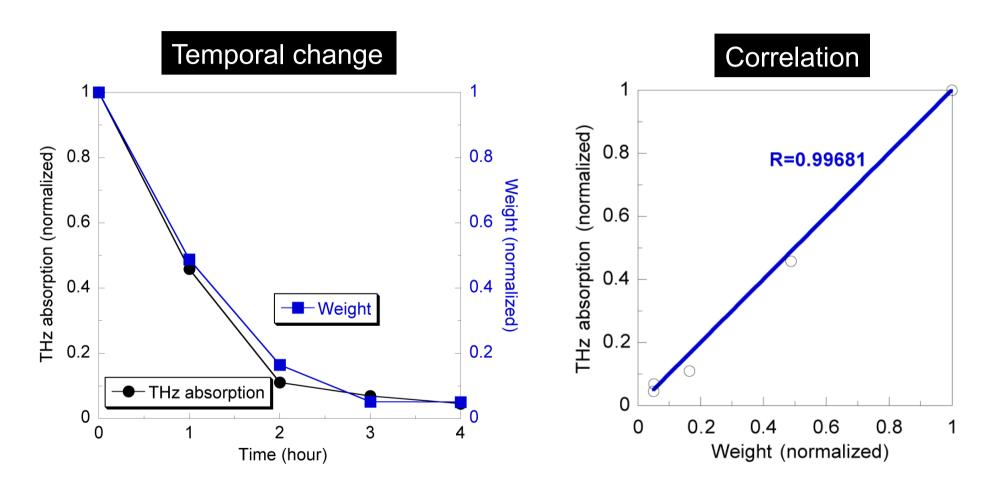
Good correlation between the two methods indicates good performance of water content measurement using THz-TDS.
