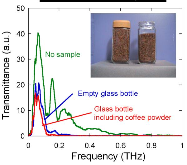
Empty glass bottle strongly absorbs THz wave > 0.1 THz because of water in the glass.
